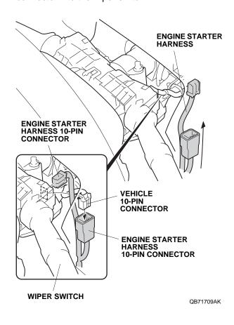
44. Align the branch point of the engine starter harness with the clip on the vehicle harness, and secure the engine starter harness to the vehicle harness using two wire ties.
