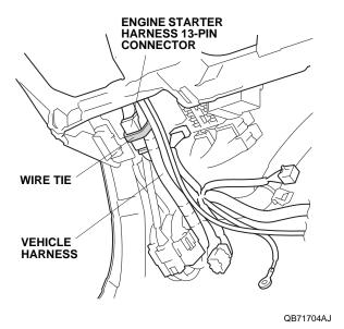
54. Attach the engine starter harness 25-pin connector to the vehicle connector as shown.
