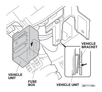
60. Unplug the vehicle 2-pin connector from the vehicle unit, and plug it into the engine starter harness 2-pin connector. Plug the remaining engine starter harness 2-pin connector into the vehicle unit.
