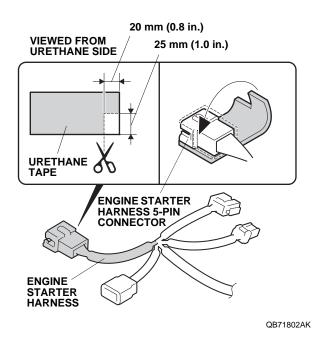
49. Unplug the vehicle 5-pin connector from the fuse box. Plug the engine starter harness 5-pin connector into the fuse box 5-pin connector. Plug the vehicle 5-pin connector into the engine starter harness 5-pin connector.
