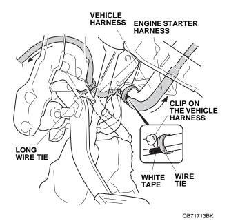
39. Using one long wire tie, secure the engine starter harness to the vehicle harness.
