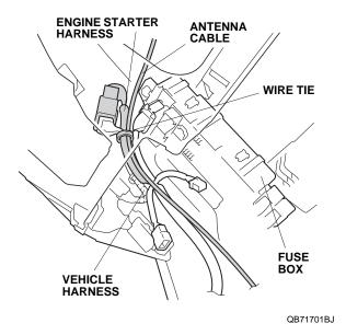
51. Plug the engine starter harness 12-pin connector into the fuse box.
