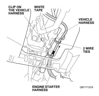
41. Using one wire tie, secure the engine starter harness to the vehicle harness.
