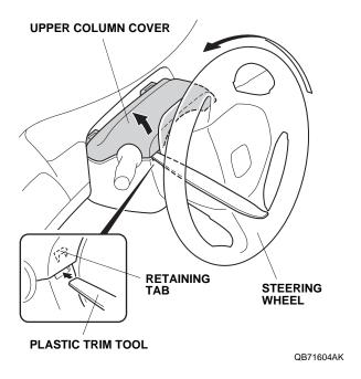
19. Turn the steering wheel 180° clockwise. Using a plastic trim tool, release the retaining tab.
