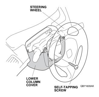
23. Remove the lower column cover (one self-tapping screw).
