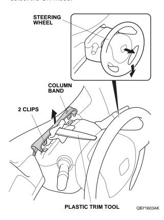
18. Turn the steering wheel 90° counterclockwise. Using a plastic trim tool, release the retaining tab.
