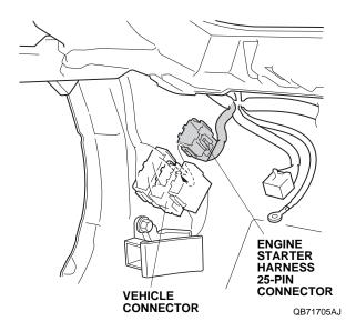
55. Unplug the vehicle 25-pin connector from the fuse box. Plug the engine starter harness 25-pin connector into the fuse box 25-pin connector. Plug the vehicle 25-pin connector into the engine starter harness 25-pin connector.
