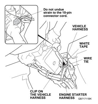
46. Using one long wire tie, secure the engine starter harness to the vehicle harness.
