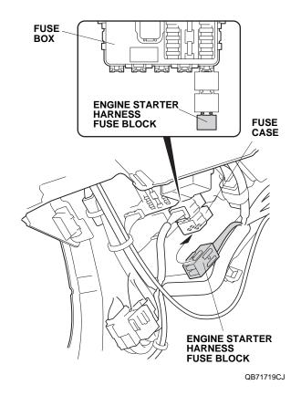
70. Using one wire tie, secure the engine starter harness to the vehicle harness.
