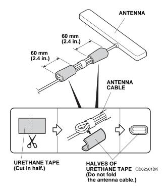
28. Starting near the antenna end of the cable, wrap two urethane tapes around the antenna cable at the measurements shown.
