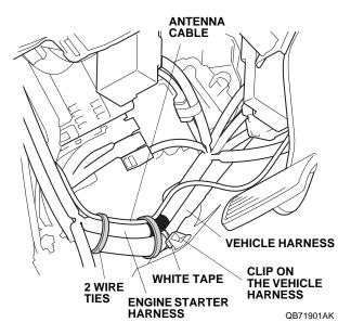
72. Using one wire tie, secure the engine starter harness and antenna cable to the vehicle harness.
