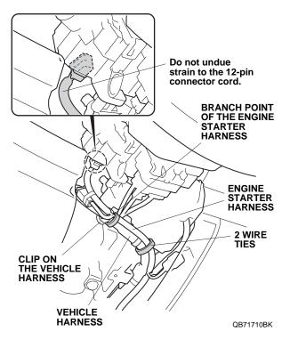
45. Align the white tape on the engine starter harness with the clip on the vehicle harness, and secure the engine starter harness to the vehicle harness using one wire tie.
