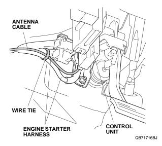
74. Bundle up the excess antenna cable as shown.
