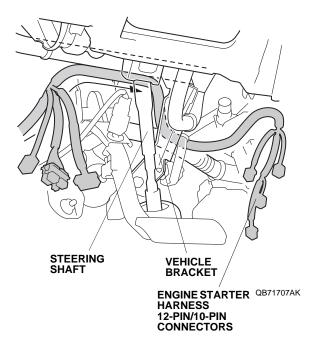
38. Align the white tape on the engine starter harness with the clip on the vehicle harness, and secure the engine starter harness to the vehicle harness using one wire tie.
