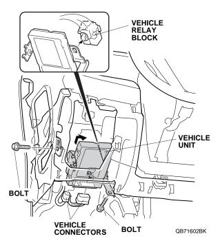
26. Remove the vehicle unit from the vehicle bracket (vehicle connectors).
