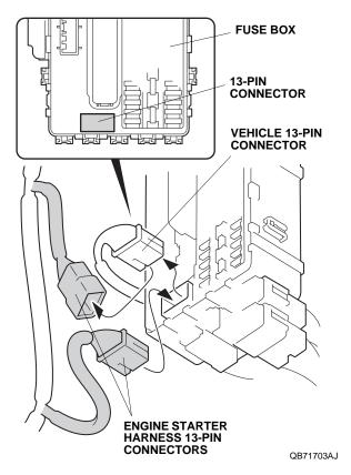
53. Using one wire tie, secure the engine starter harness 13-pin connector to the vehicle harness.
