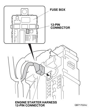
52. Unplug the vehicle 13-pin connector from the fuse box. Plug the engine starter harness 13-pin connector into the fuse box 13-pin connector. Plug the vehicle 13-pin connector into the engine starter harness 13-pin connector.
