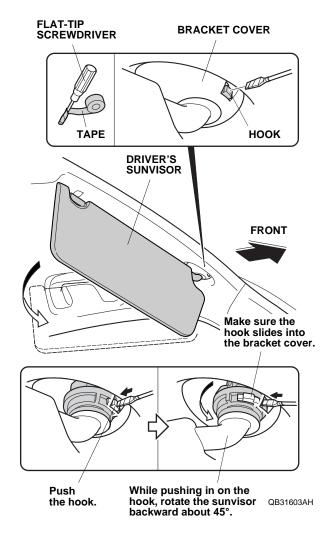
6. While pushing in on the hook, rotate the driver's sunvisor backward about 45°. Make sure the hook slides into the bracket cover.
