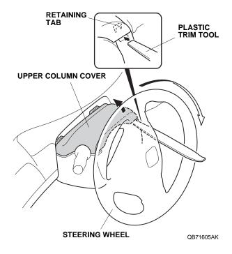
20. Remove the upper column cover (two retaining tabs and two hooks).
