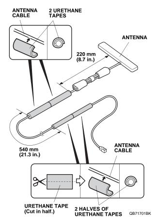
29. Using scissors, cut one urethane tape in half. Wrap the two halves of urethane tape around the antenna cable at the measurements shown.
