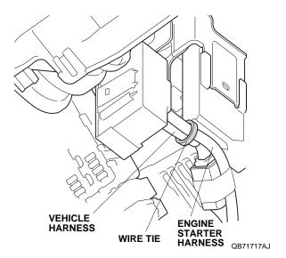
71. Align the white tape on the engine starter harness with the clip on the vehicle harness, and secure the engine starter harness and antenna cable to the vehicle harness using one wire tie.
