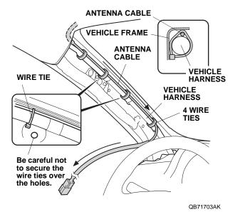
33. Pull away the door opening seal. Route the antenna cable down and under the dashboard through the driver's A-pillar trim opening.
