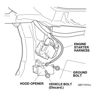
57. Using one wire tie, secure the engine starter harness to the vehicle harness.
