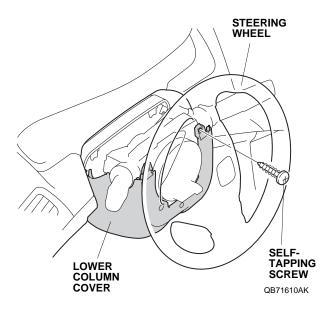
22. Turn the steering wheel 180° counterclockwise, and remove the other self-tapping screw from the lower column cover.
