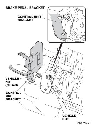
66. Using a felt-tip pen, mark the control unit bracket and vehicle nuts.
