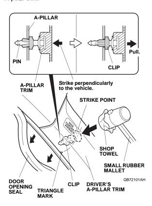
9. Using a small rubber mallet and a shop towel, gently tap the driver's A-pillar trim at the position shown to release the clip.
