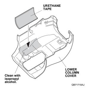
78. Attach the urethane tape to the lower column cover in the area as shown.
