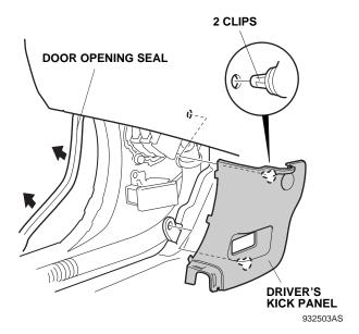
16. Pull away the door opening seal, remove the driver's dashboard side lid (three clips, four pawls, and three hooks).
